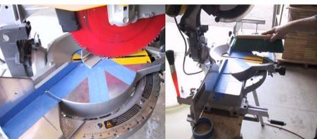
Tape the face of the saw surface to avoid damage such as marring the surface of Edge Trim. As shown above
